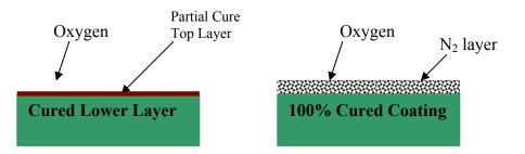
A less than fully polymerized coating can be a sticky matter. The topmost layer of the coating being tacky and lacking surface properties needed in the final product. If the surface is wiped with solvent to remove this top layer (frequently 5% or less of the film thickness, the coating can be fully cured below (where no ambient oxygen was present to cause inhibition.
