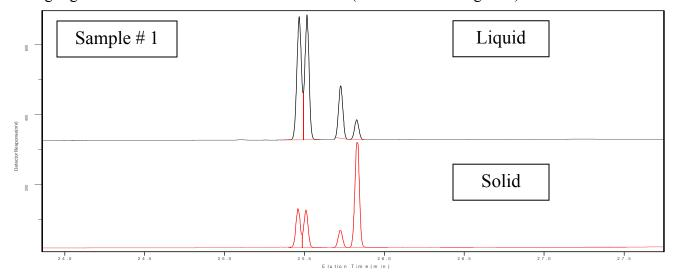
Figure 2: GC scans for the liquid and solid phases of Sample #1 (upper GC: liquid sample; lower GC: solid sample). The isomer elution sequence is cis-1,3-; trans-1,3-; cis-1,4-; trans-1,4- as determined by NMR. The trans-1,4diacrylate is the minor isomer in the liquid sample and the major isomer in the solid sample.
