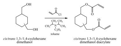
Figure 6: Acrylation of 1,3/1,4 CHDM with acryloyl chloride in toluene.
