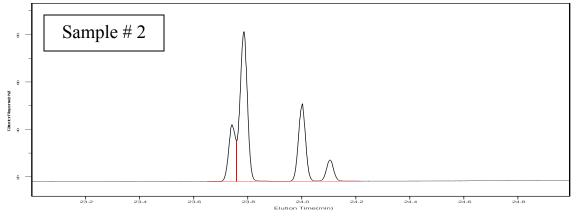
**Figure 3**: GC scans for liquid cyclohexanedimethanol diacrylate (Sample #2). The isomer elution sequence is the same as in Figure 2.
