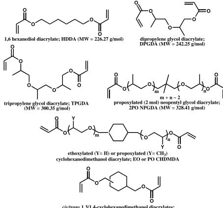
*cis/trans* 1,3/1,4-cyclohexanedimethanol diacrylates; 1,3/1,4 CHDMDA (MW = 252.31 g/mol)
