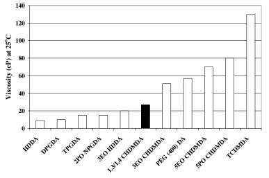
Figure 7: Viscosity comparison of diacrylate monomers
