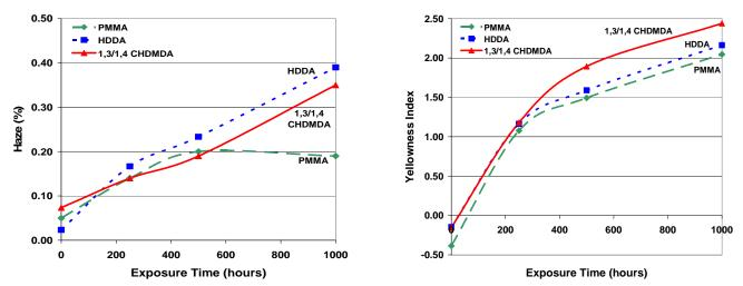
Figure 8: Effect of QUV exposure time on haze and yellowness index of UV coatings applied on PMMA.
