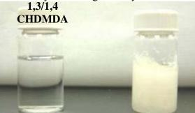
Figure 4: Appearance of liquid 1,3/1,4 CHDMDA (left) vs. solid 1,4 cyclohexanedimethanol diacrylate (right).
