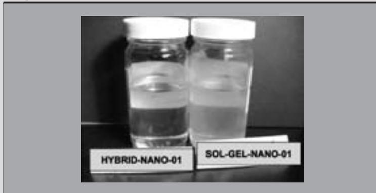
After nanoparticle surface modification, the nanoparticles can be dispersed in desired UV resins and co-cured. This proprietary surface-treatment technology enables low viscosity, even at relatively high nanoparticle loadings and overcomes Rayleigh scattering issues for optical transparency (see Figure 2 and Table 4).
