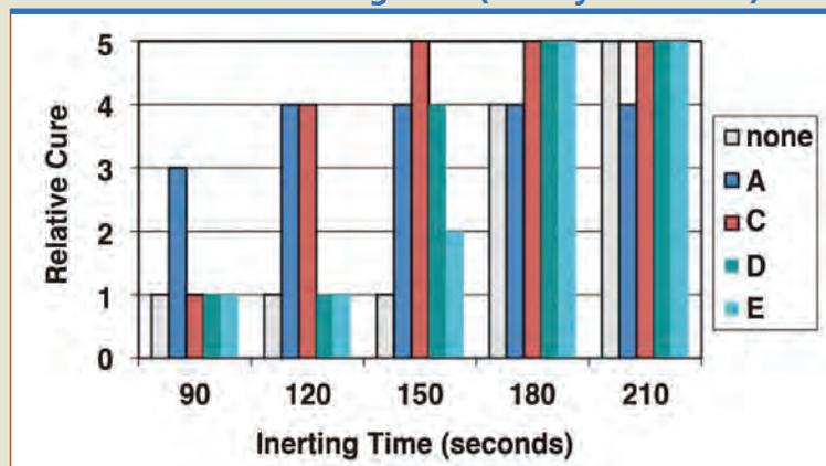
by starting the EB system with the reaction chamber in an air atmosphere. A nitrogen purge was then started at a low flow rate of 18 scfm. Coating samples were then irradiated at 30-second intervals while continuing the purge. This produced an oxygen concentration gradient that decreased with increasing purge time. The actual oxygen concentration at the time of irradiation could not be measured due to the lag time in the response of the electrochemical oxygen sensor used in the EB system.
