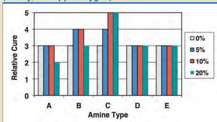
with no remaining acrylate functionality C; acrylated amine with both amine and acrylate functionality D; and an amine modified oligomer E. An amine zirconate complex B was also tested.
