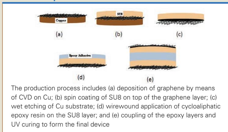
based polymer electrode.<sup>6</sup> A graphene to SU8 epoxy polymer transfer method was established. This transfer technique consists of coupling the graphene layer to a supporting polymer before a chemical etching of the catalyst is performed, in order to release the supported graphene from the synthesis substrate.
