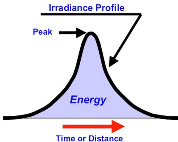
**FIGURE 1.** Illustration of irradiance profile, peak irradiance and energy
