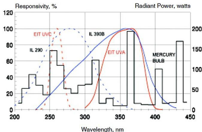
**FIGURE 2.** Selected examples of radiometer spectral response and mercury lamp emission
