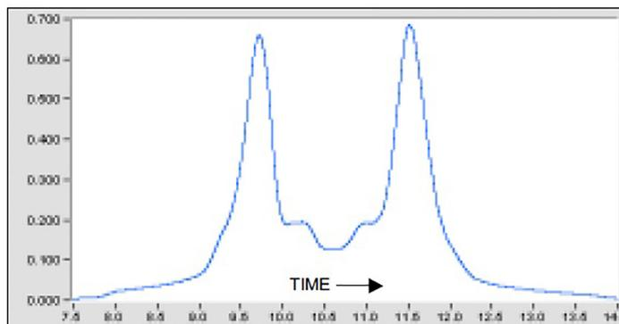
**FIGURE 3.** Irradiance profile of two lamps (rows) in sequence
