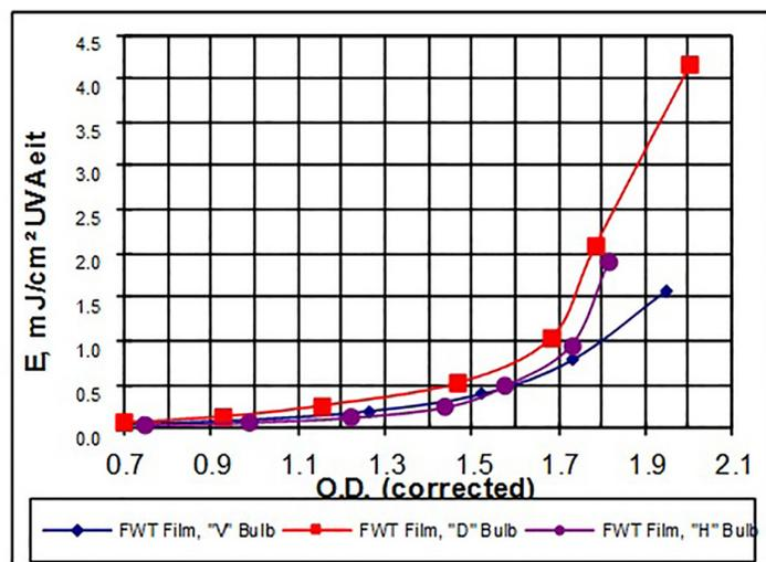
**FIGURE 4.** Correlation of radiachromic film with various medium-pressure bulbs
