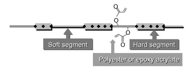
Fig. I: Building blocks of UV-curing polyurethane dispersions
