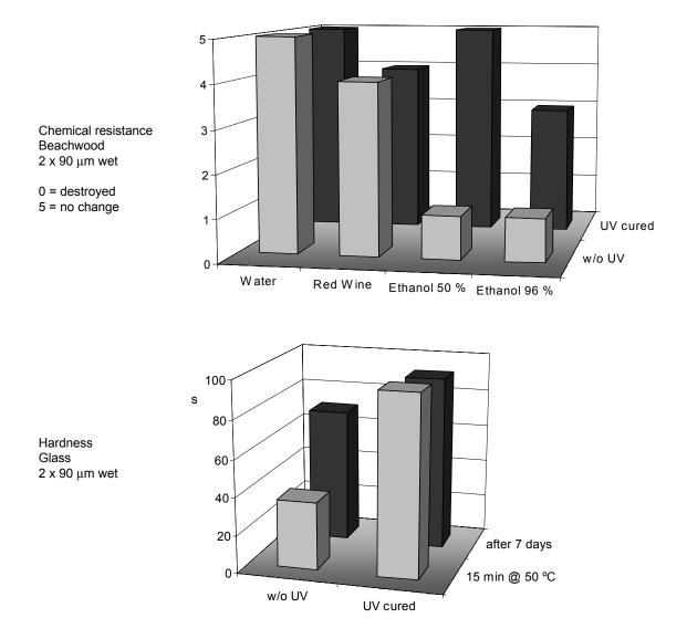
**Fig. II**: Chemical resistance and hardness of PU dispersion-based, white pigmented coating with and without UV-curing.
