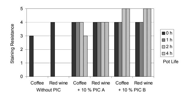
**Fig. III**: Staining resistance of dual cure waterborne UV pigmented coatings DIN 68861 1b, 5 = pass, 0 = fail
