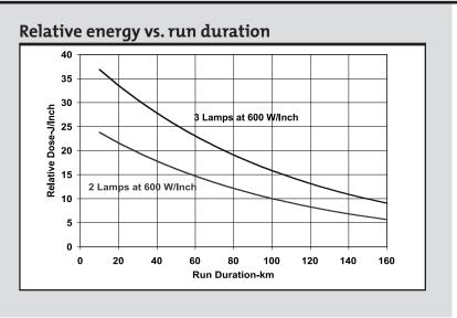
The minimum value of relative energy must now be determined to assure adequate colored fiber cure.
