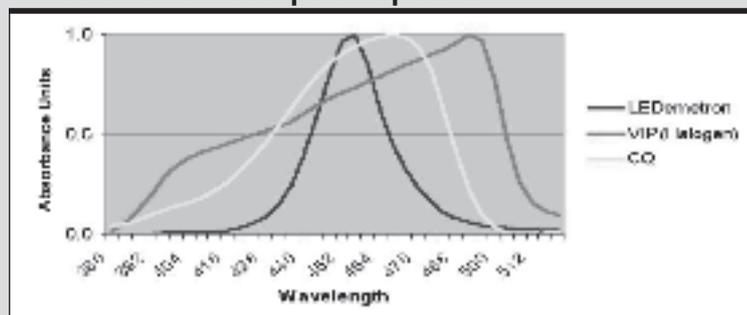
Spectral output of LED matches absorption characteristics of photoinitiator *d,l* camphorquinone (CQ). Halogen lamps may also work, but are not as effective.
