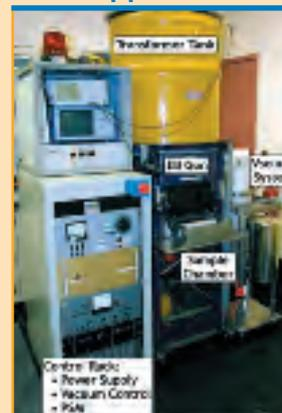
$V_c$  and  $V_b$  are both measured using an oscilloscope. In this manner, if the charge collector's signal is initially calibrated against a radiochromic chemical dosimeter, the inferred dose per pulse can be continuously monitored.
