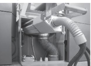
Gear-side view of interstation UV-curing unit from below.
