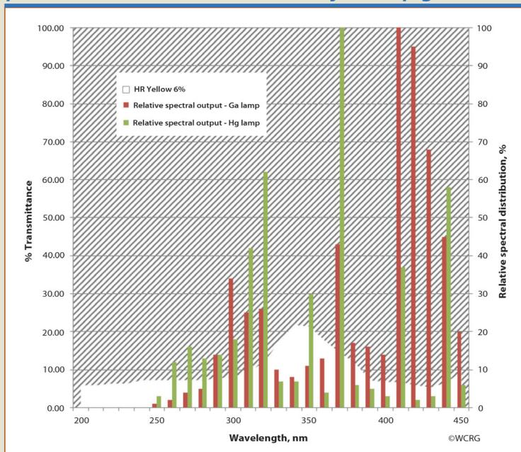
these parameters will result in reduced cure and performance. When utilizing pigments in UV-cured coatings, it is important to understand that only a certain amount of light will be available for curing.
