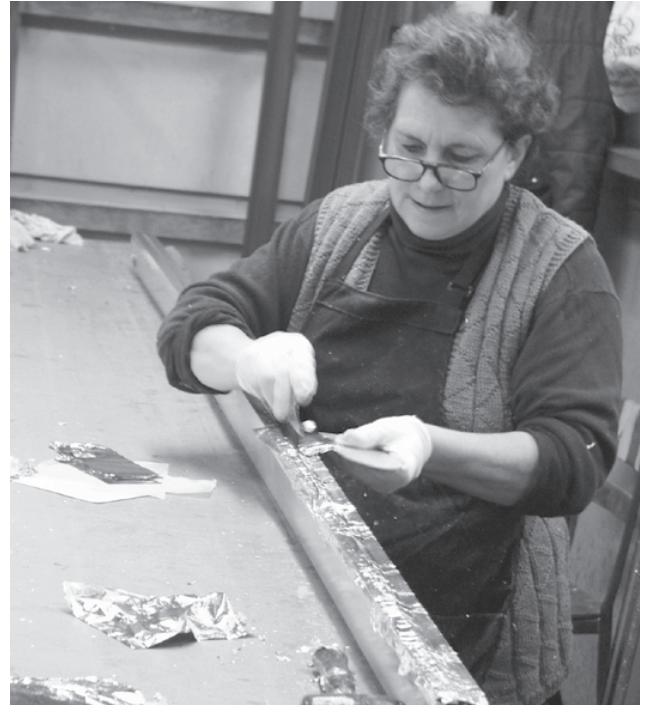
PB&H specializes in hand finishing, but a UV clearcoat was an excellent solution to a big bottleneck.
