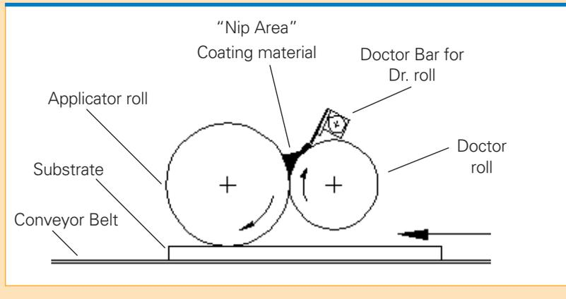
Standard application rollers can apply about 1 mil of film thickness without having a streaked appearance.
