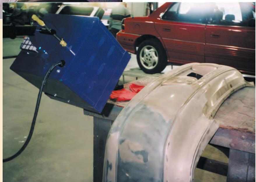
*A low-energy lamp is used to cure the primer.*
