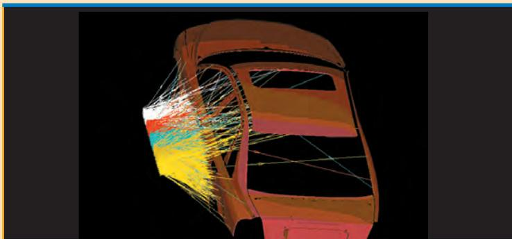
A CAD representation of the physical dimensions and components of the UV-curing area in the finishing line is required. The software uses this data when analyzing the movements of the lamps to assure that they will not collide or interfere with other components in the area. Other important variables that are needed relating to the finishing line are the line speed, starting position of the UV lamps, and position of the target relative to the UV lamps.
