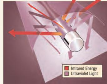
*CoolWave system emits up to 30% less infrared energy than conventional microwave UV systems.*
